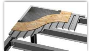
Checker plate on OSB and roof deck
