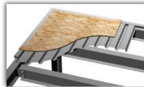
OSB and roof deck
