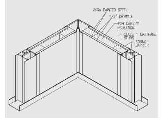
Note: An STC rating identifies the sound transmission class for the panel only. For the best sound solutions you must consider the entire structure.
