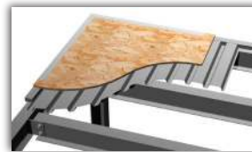
OSB and roof deck
