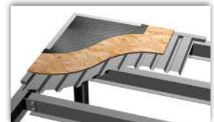
Checker plate on OSB and roof deck
